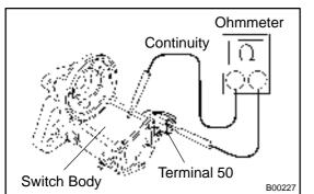
(b) Check the hold-in coil for open circuit. Using an ohmmeter, check that there is continuity between terminal 50 and the switch body.
