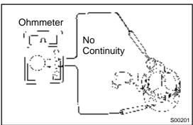
(b) Check for field coil for ground. Using an ohmmeter, check that there is no continuity between the field coil end and field frame.
