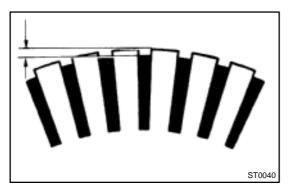
(c) Check that the undercut depth is clean and free of foreign materials. Smooth out the edge.
